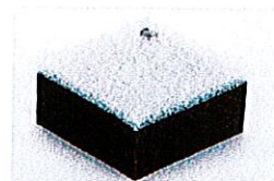
Packaging Foam bonded to EVA Foam
