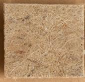
Eco Friendly Jute Fiber Recycleable 3D Fold or Mold - Build Your Composite 3D Pressing at 250°F - 400°F Stackable, Tackable, Acoustic, and Deco
