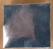
Reflective Foil & Polyester ES - 403 .125" Maximum Thickness - Waterproof - Sewable .005" Foil Outer Layer (1-side) .120" Polyester "Loft" - Spot Sonic Welded
