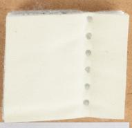
Energy Saver Select ES - 401 .200" Thick (at full fluff) - Foils and Cottons Polyester-Deco Outer Layers Available Spot Sonic Welded - 6 Layer
